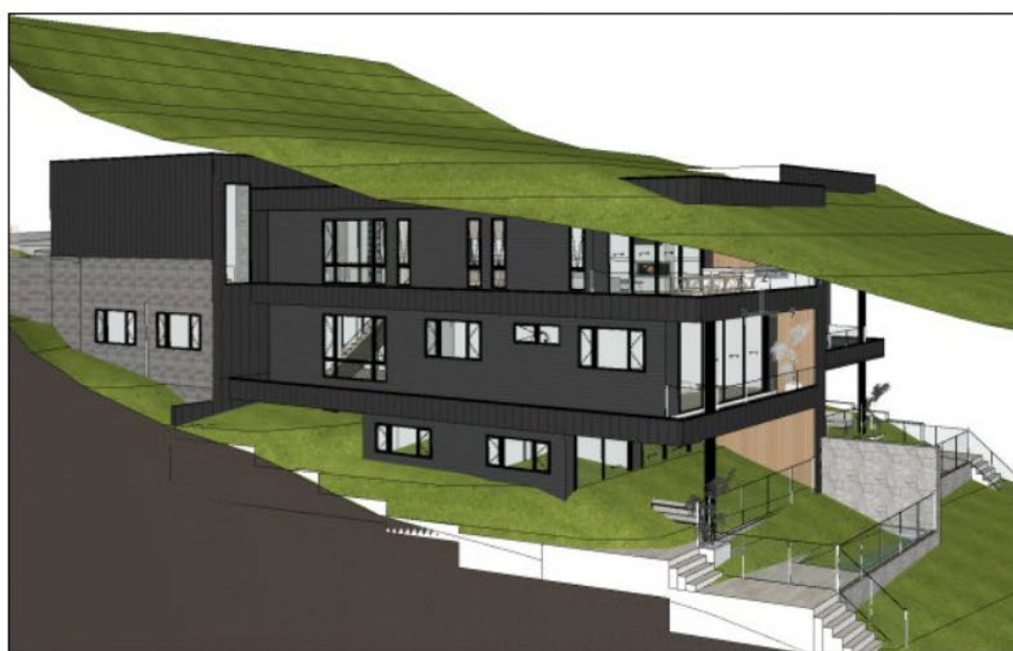
Figure 4: 3D model of the proposed development with the natural ground level and 9m height limit shown by the green plan to identify areas of the height exceedance
