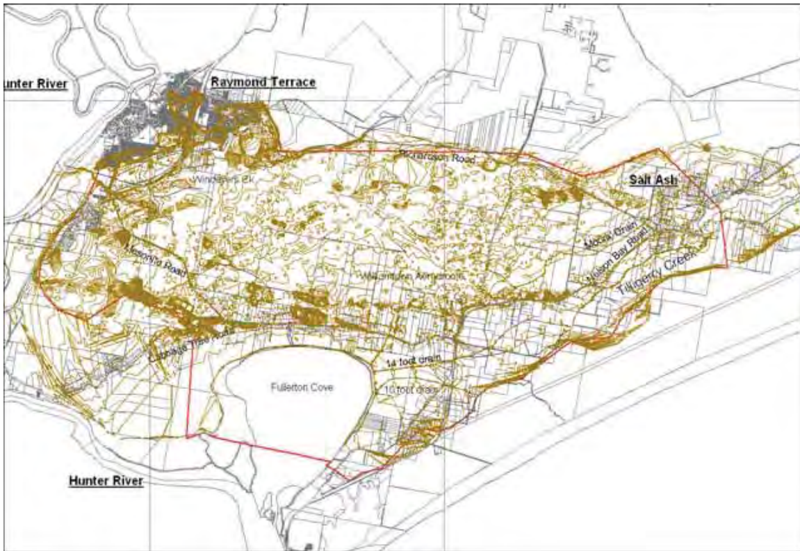
Figure 4-2 1m contour lines of the DTM in the project area
