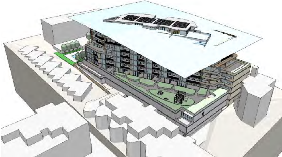
Figure 1: The blue plane represents the 28m LEP height standard. The area above exceeds the height limit, which consists mainly of the covered communal and private open space for residents, primarily at the northern portion due to the cross fall of the site.
