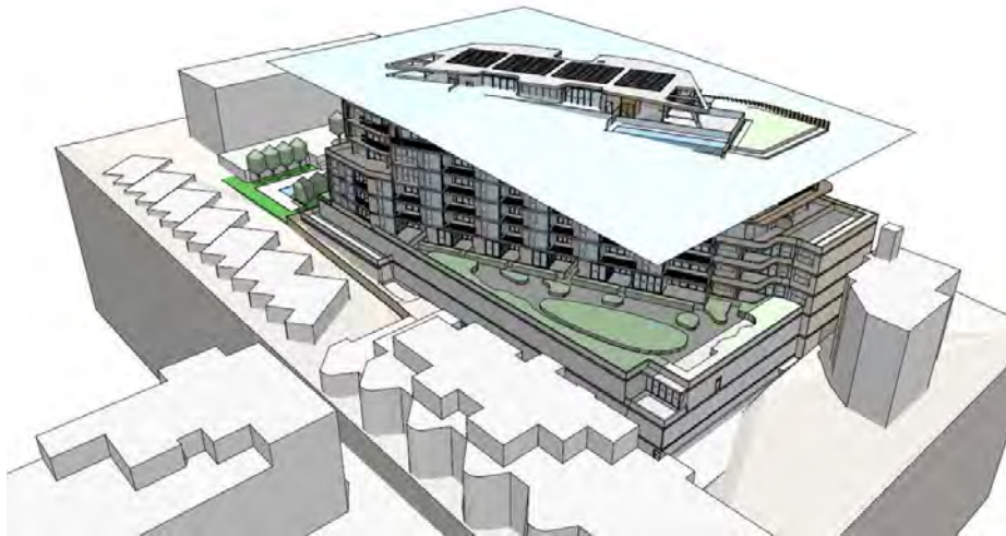
Figure 1: The blue plane is 28m above ground. The area above exceeds the height limit, which consists mainly of the covered communal and private open space for residents.
