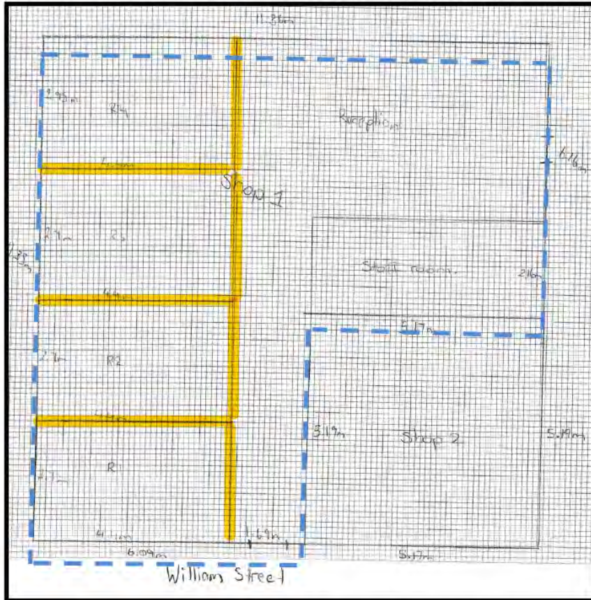
Figure 1 – Proposed internal fit out floor plan. Proposed walls highlighted in yellow. Shop boundary lines in blue.
