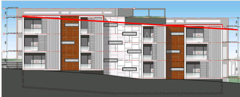
Figure 5 – Plan extract of northern façade showing 9m height breach (in red).
